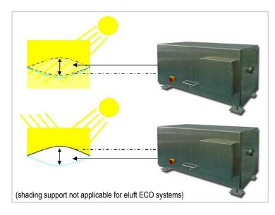
The shading controls are integrated in the eluft unit and make sure that the air needed to move the middle layer is taken from the chambre which becomes free from air. As the air flowing to shade the pillows does not need to be dried, it becomes more energy-efficient.
